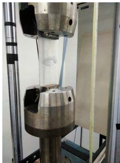
Figure 3.8: Aluminium plate was clamped into the UTM jigs.
