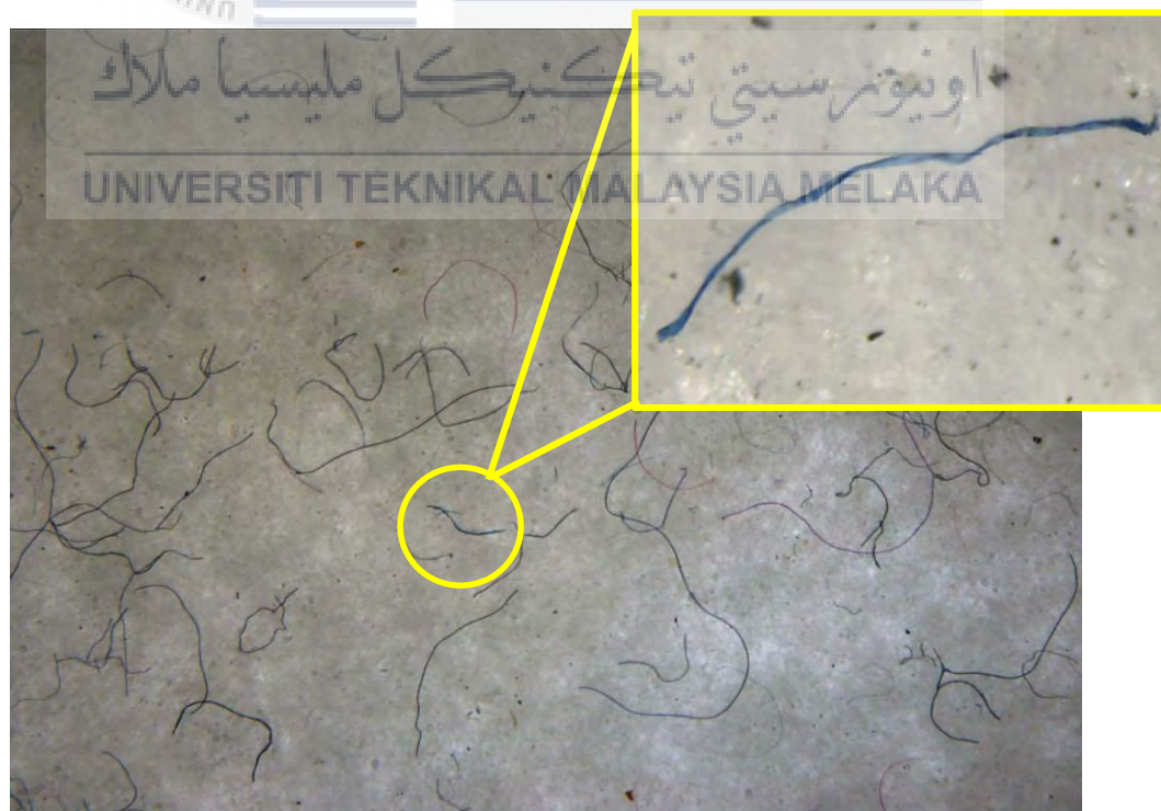
Figure 4.12 Visual microscopic observation of fibers extracted from oil sample
