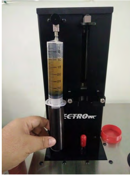
Figure 3.20 Insertion of large syringe to the top chamber
