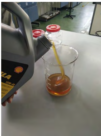
Figure 3.6 Pour of 500 ml engine oil into a beaker
