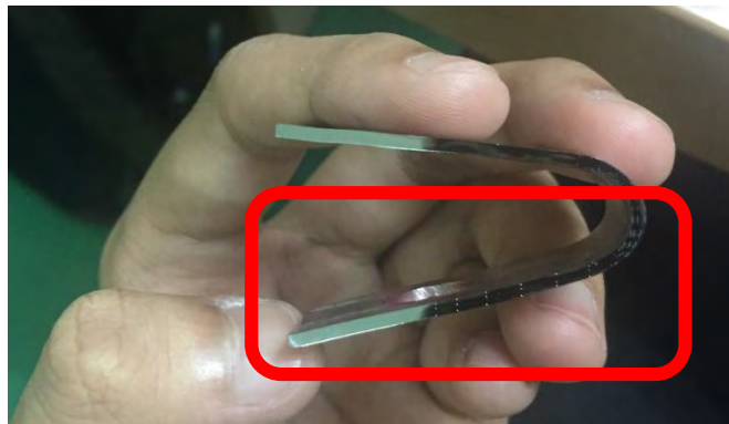
Figure 4.31: Indentation marks from region 1 to 9 in specimen 1.4 mm
