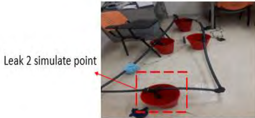
Figure 4.6: Leak 2 simulation point
