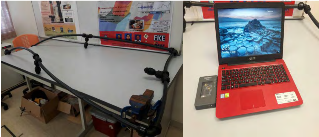
Figure 3.5: Project setup between sensor, pipe, NI myRIO-1900 and Host Computer
