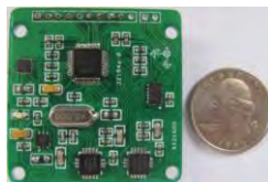
Figure 2.7: Physical structure of AHRS module [22]
