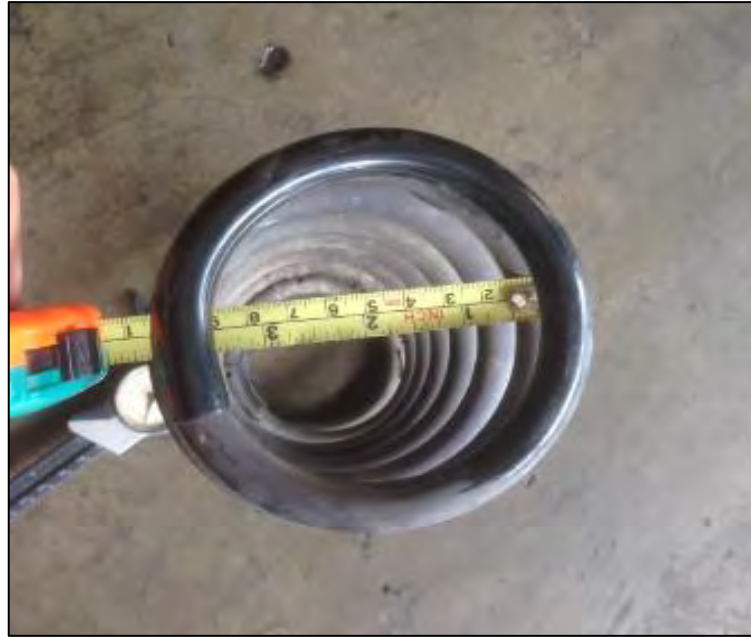
Figure 3.4: Measurement of spring diameter
