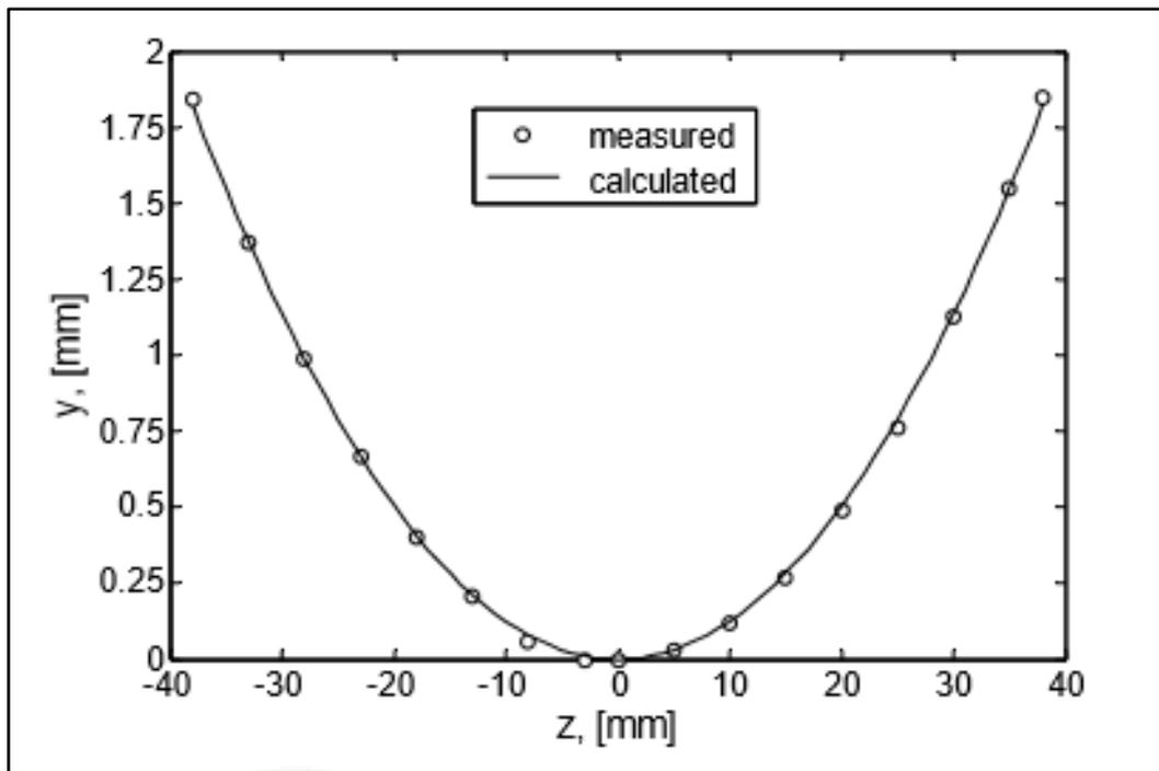
Figure 2:3 : Elastic line of sample.
