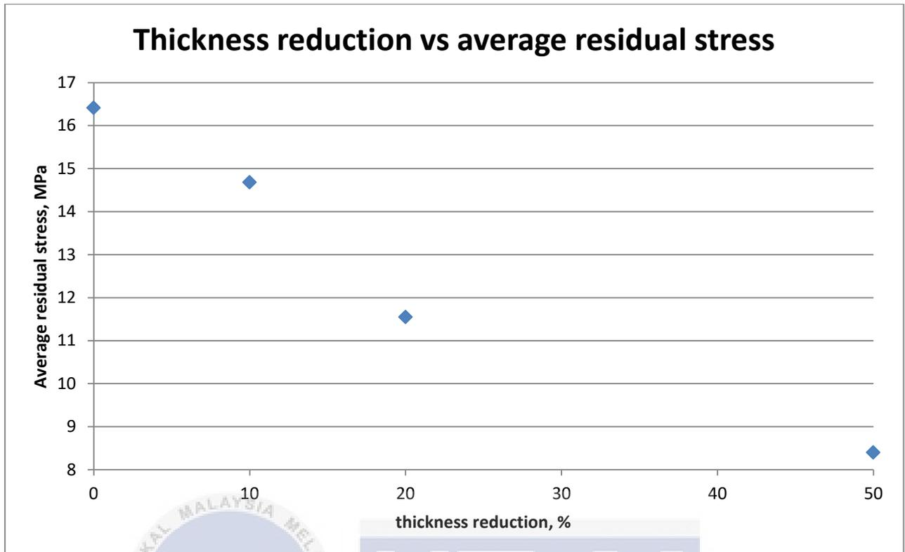
Graph 5:3 Thickness reduction versus average residual stress.
