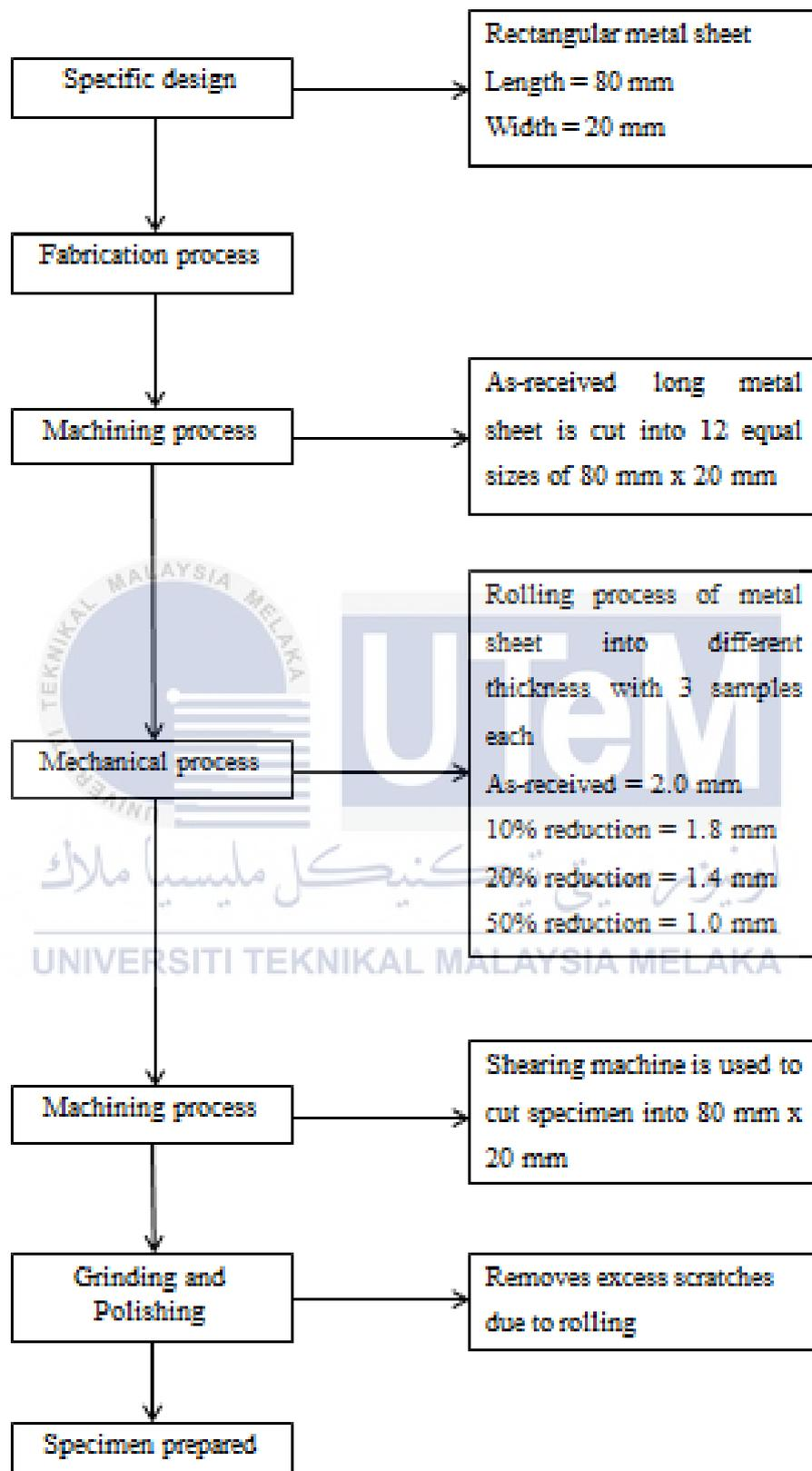
Figure 3:2 Flowchart of specimens preparation.
