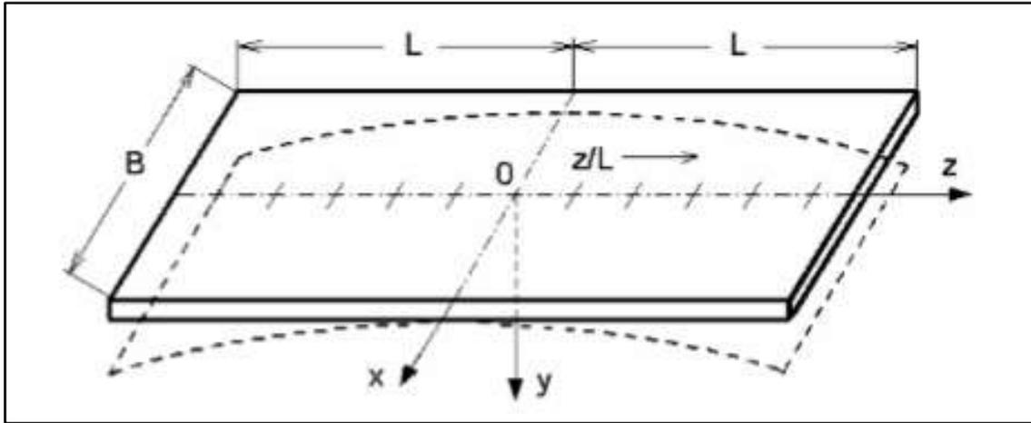
Figure 2:2 : Schematic presentation of elastic bending under influence of residual stress.
