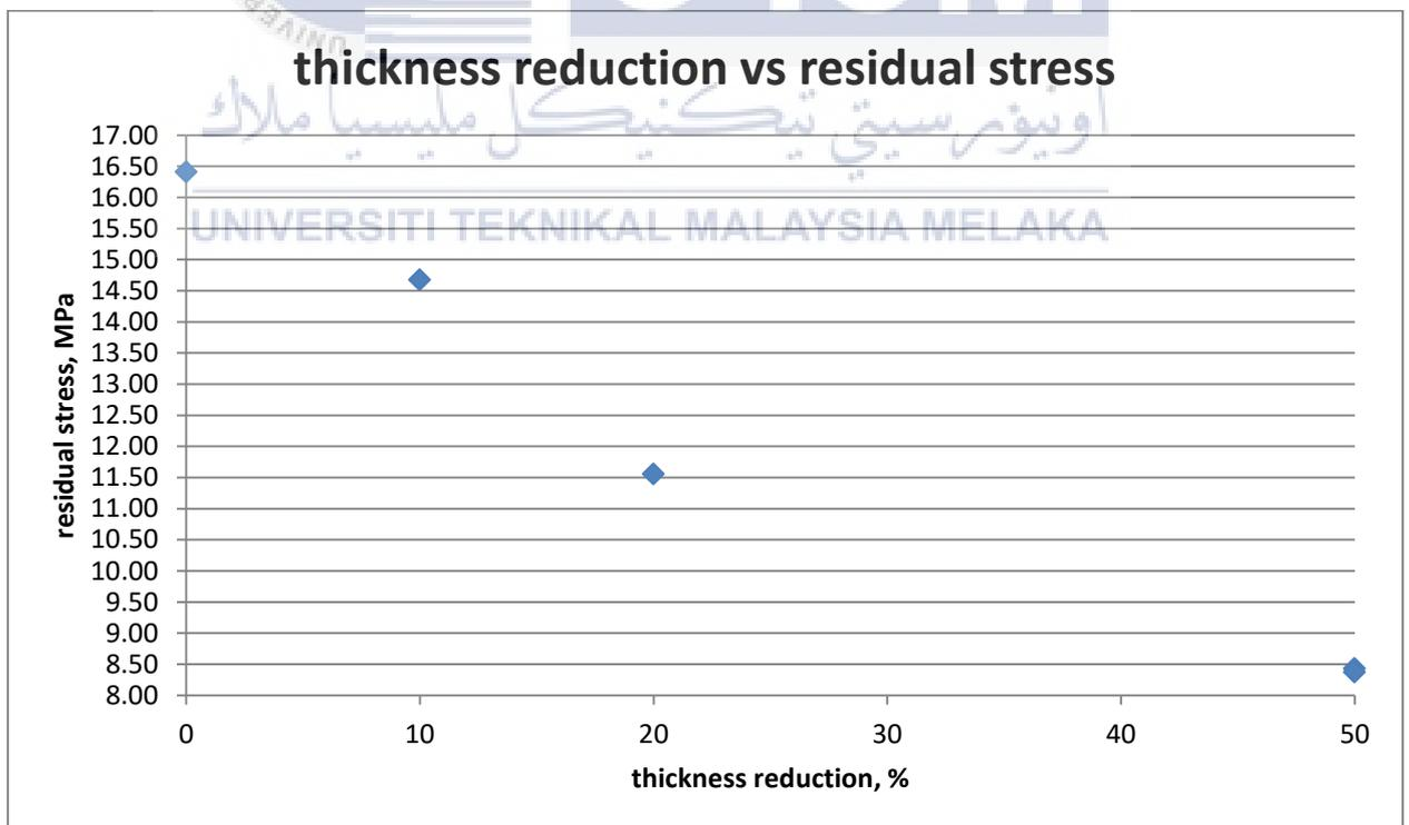
Graph 5.2 Thickness reduction versus residual stress.
