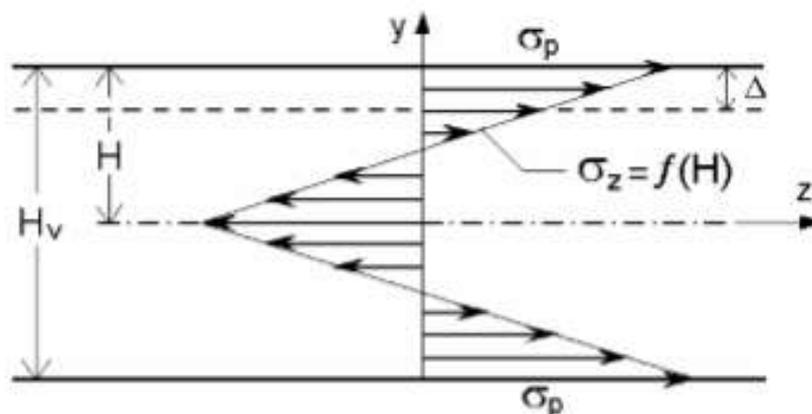
Figure 5:1 Overview and parameters used for residual stress calculation.
