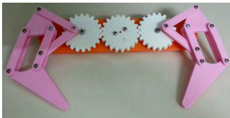
Figure 3.13: Gear and linkage construction
