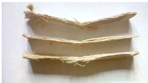
Figure 3.12: Specimen after the flexural test
