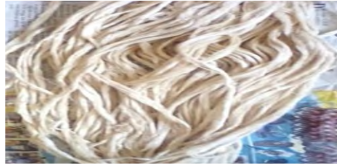
Figure 3.4: The PLF after undergone the process of removing the excess lignin and cellulose
