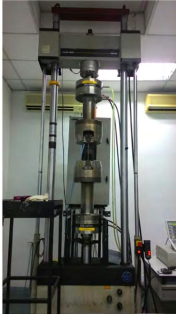
Figure 3.7: Instron Universal Testing Machine
