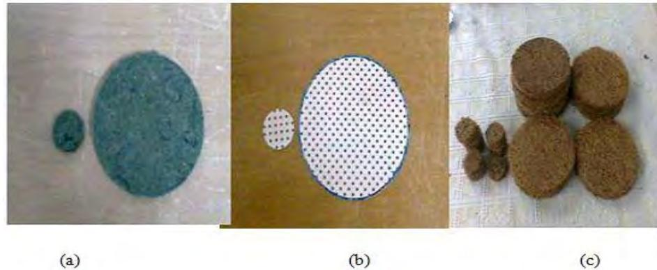
Figure 2.8: Test samples (a) porous layer (b) perforated panel (c) coconut coir fiber
