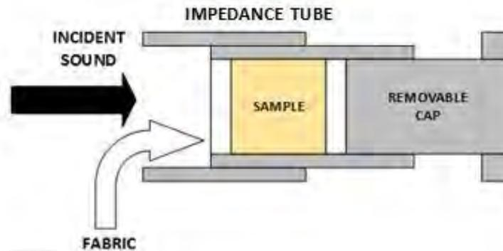
Figure 4.4: The setup for rigid backed added with fabric at the front and back of the sample in the impedance tube
