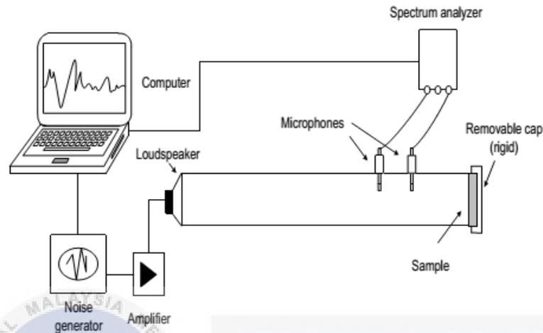
Figure 3.12: Experimental setup for sound absorption coefficient test (Putra et al., 2013)
