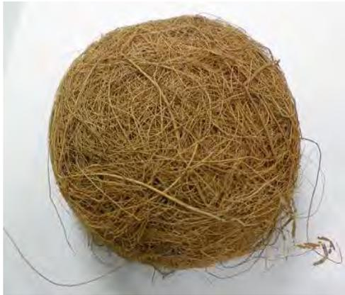
Figure 2.6: Coir fiber in disk form Fouladi et al., (2013)
