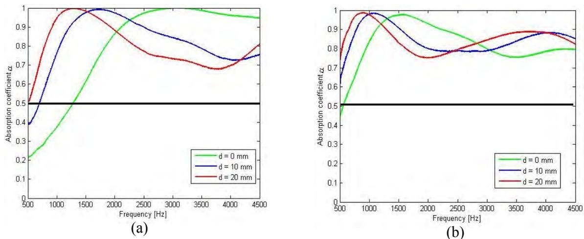
Figure 4.9: Measured sound absorption coefficient of PLF fibers with different air gaps (a) 20 mm thickness (b) 30 mm thickness
