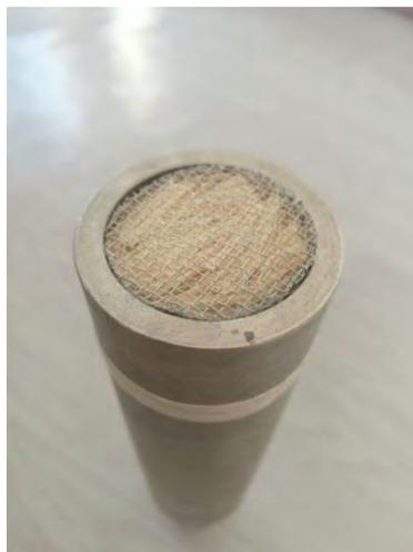
Figure 3.13: Sample PALF fitted in the sample holder
