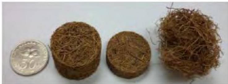
Figure 2.11: The samples of oil palm fiber (Or et al., 2015)
