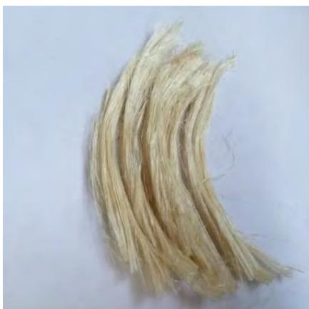
Figure 3.6: The pineapple leaf fiber after treatment process
