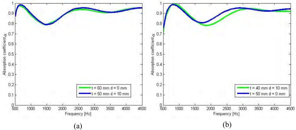
Figure 4.13: Comparison of sound absorption coefficient between samples with thickness (a)  $t = 50 \text{ mm} + d = 10 \text{ mm}$  and  $t = 60 \text{ mm}$  full thicker (b)  $t = 40 \text{ mm} + d = 10 \text{ mm}$  and  $t = 50 \text{ mm}$  full thicker at the same PALF density of  $116.92 \text{ kg/m}^3$
