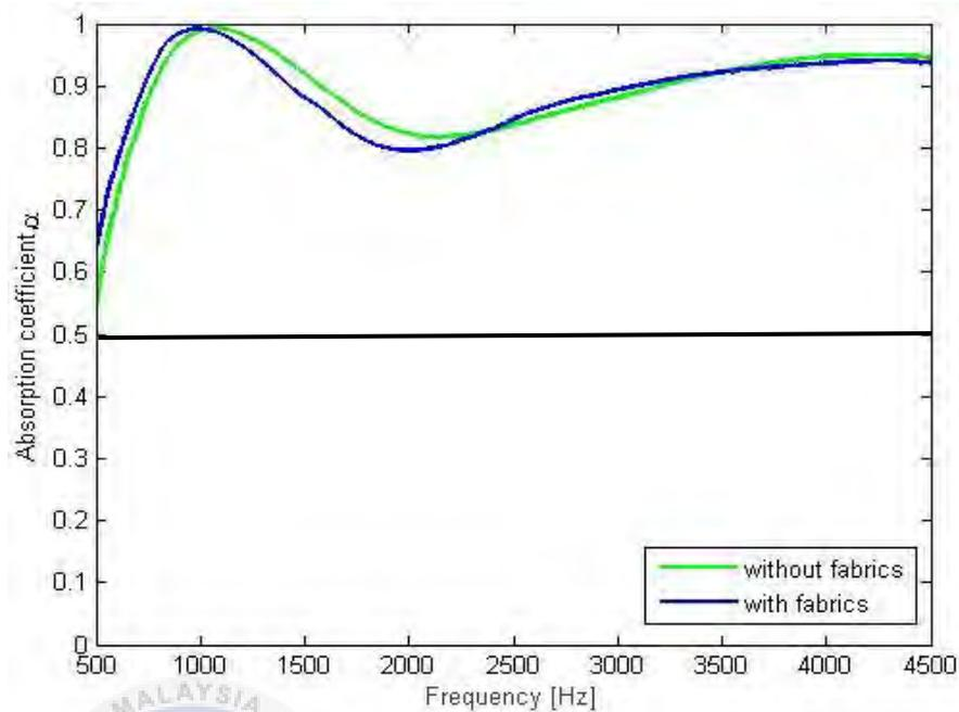
Figure 4.7: Measured sound absorption coefficient of PLF fibers with 4 cm thickness added with fabric at front and back of samples.
