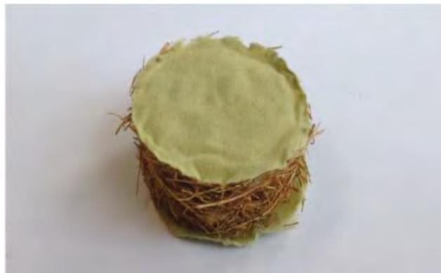
Figure 2.12: Sample of the paddy fiber attached with polyester fabric
