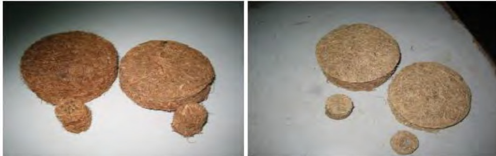
Figure 2.5: Test samples of date palm fiber (left) and oil palm fiber (right) (ALRahman et al., 2014)
