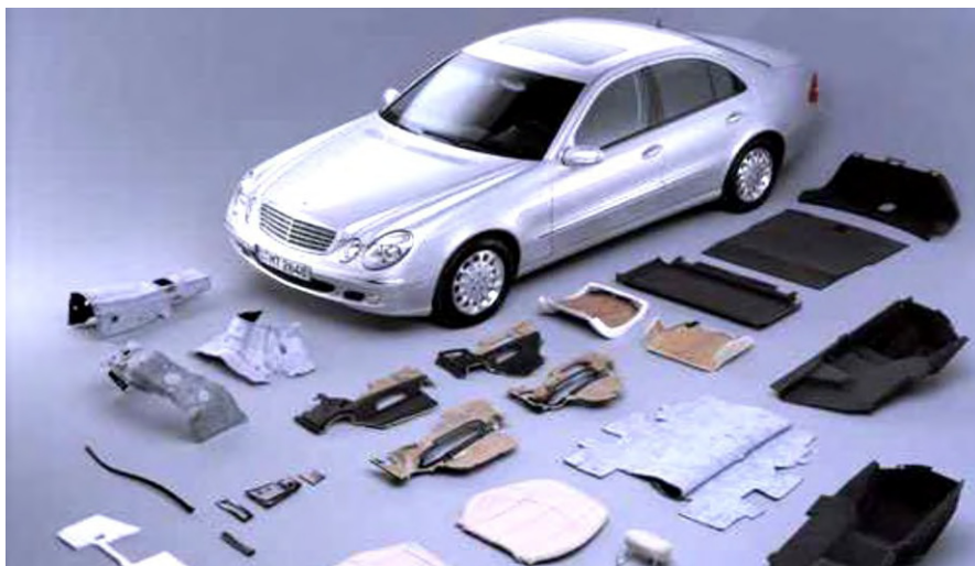
Figure 2.2: Automotive body part made of natural fiber (Monteiro et al., 2011)
