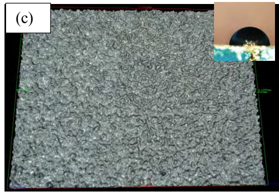
Figure 4.10: (a), (b), and (c) Surface morphology for difference time exposure to heat treatment 10, 20 and 30 minutes.
