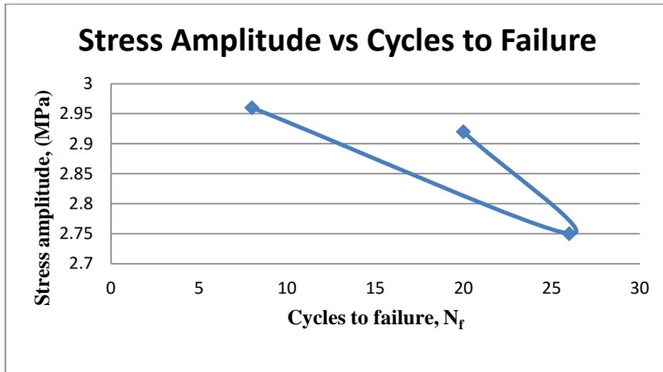
Figure 4.6: Stress amplitude versus cycles to failure for 80% stress level
