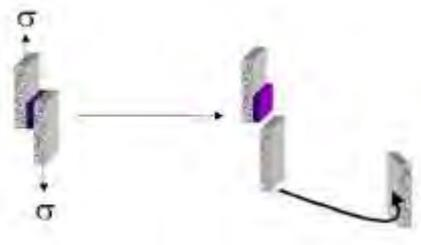
Figure 2.5: Adhesive Failure Mode (Adhesives.Org and Sealants.Org, n.d)
