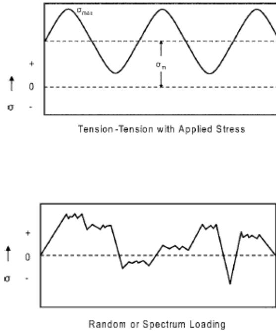
Figure 2.11: Types of Fatigue Loadings (ASM International, 2008)
