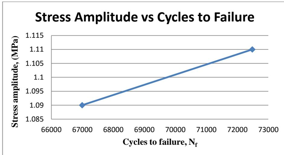
Figure 4.10: Stress amplitude versus cycles to failure for 30% of stress level
