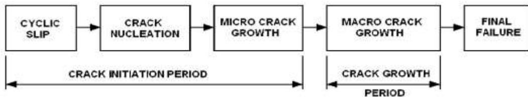
Figure 3.6: Phases of fatigue life (Azeez.A.A, 2013)
