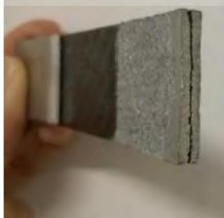
Figure 5.4: Debonding of carbon laminate composite
