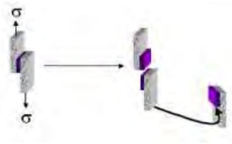
Figure 2.4: Cohesive Failure Mode (Adhesives.Org and Sealants.Org, n.d)
