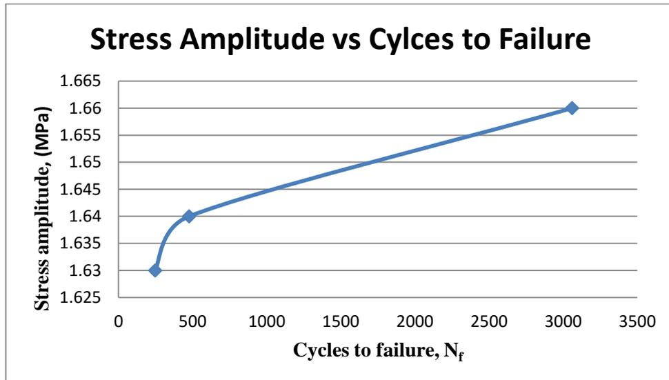
Figure 4.8: Stress amplitude versus cycles to failure for 50% of stress level
