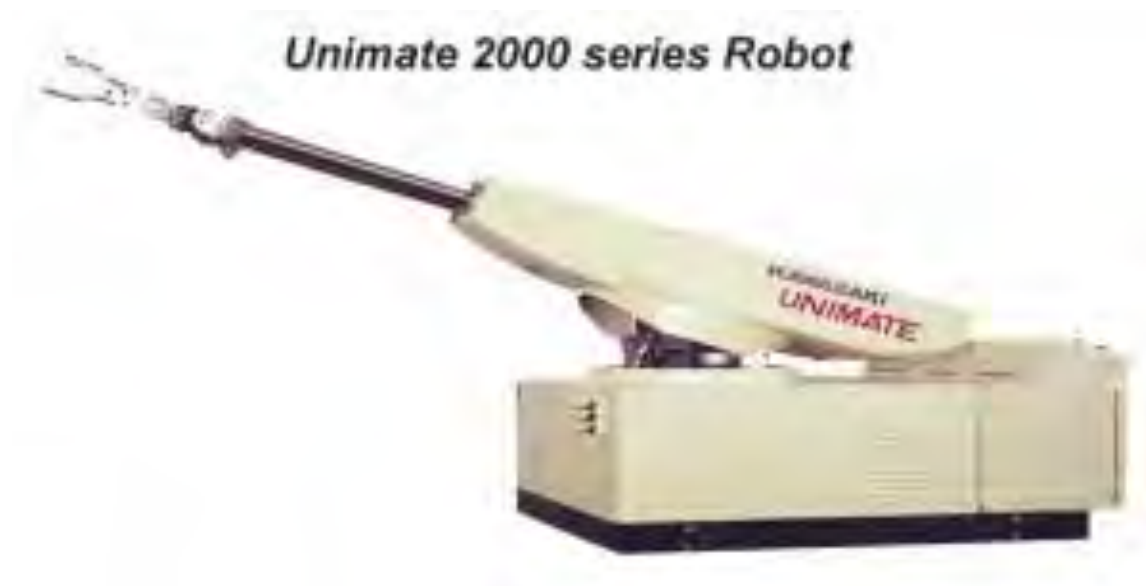
Figure 2.2: UNIMATE Polar configuration robot (Source: Robotics Bible, 2011)
