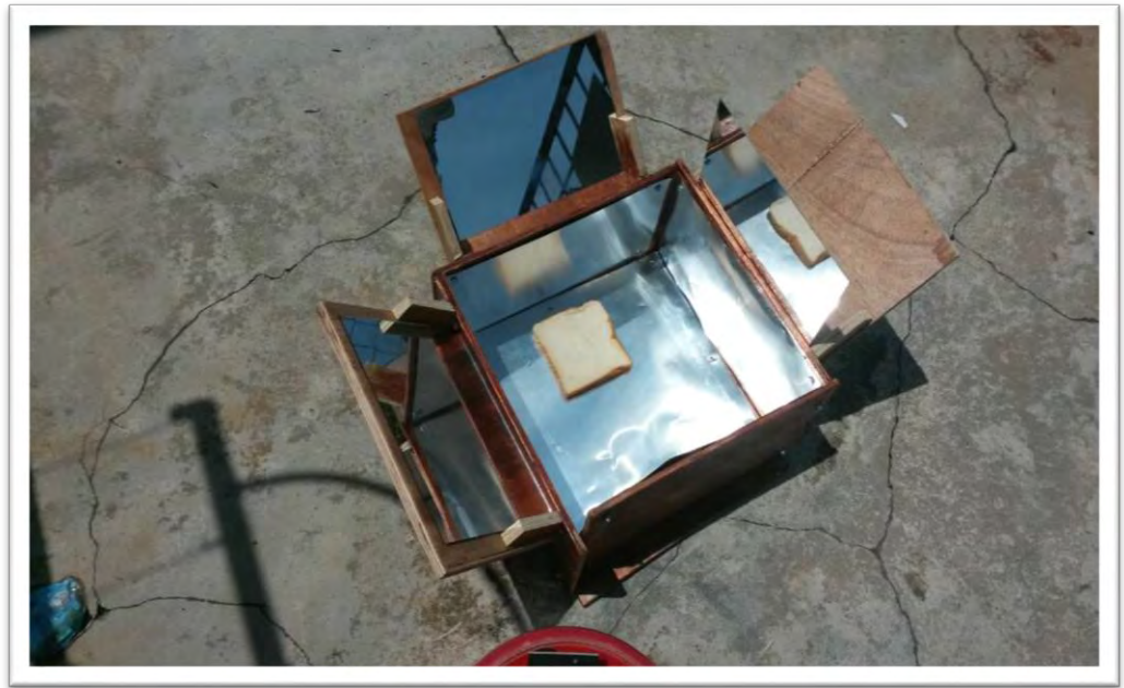
Figure 5.2 : Prototype of solar toaster been tested.
