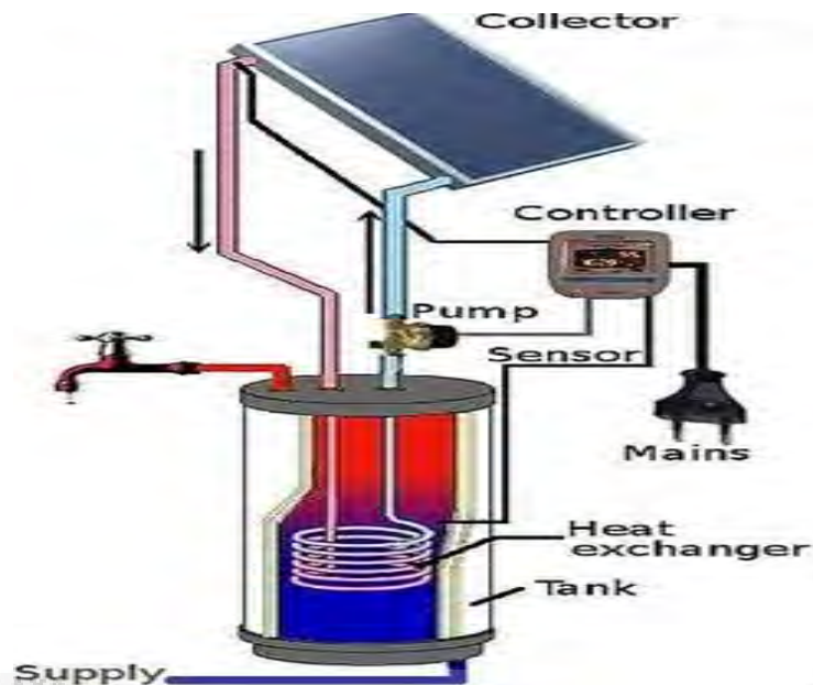
Figure 2.13(a): Domestic water heating mechanism, Diagram ( Without reservoir )
