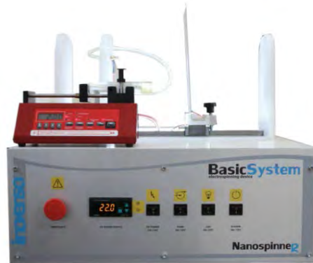
Rajah 2.8 : Pemintalan Electric The Stand-Alone Basic
