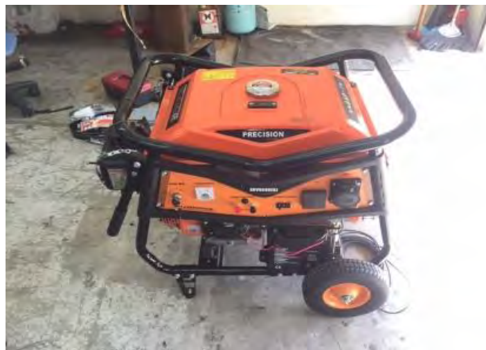
Figure 3.3: Generator engine model single cylinder
