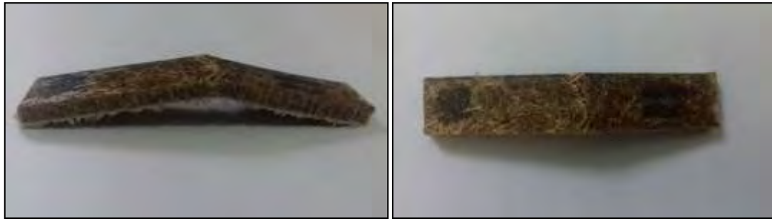
Figure 4.61 Sample 100% OPEFB fracture results
