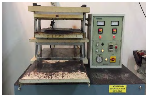
Figure 3.4: Hydraulic Hot Molding Machine.
