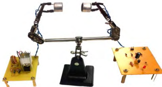
Fig. 9: AET basic system using push-pull power converter transmits energy through the air medium.
