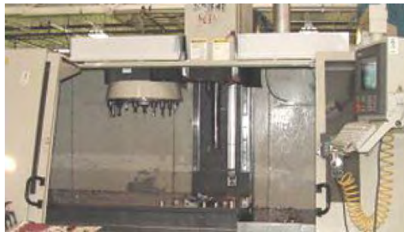
Figure 1.1: A CNC mill, often called a machining center, holds a part while a rotating tool cuts metal.
