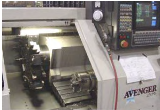
Figure 1.2: A CNC lathe, often called a turning center, rotates a workpiece while a tool cuts metal.
