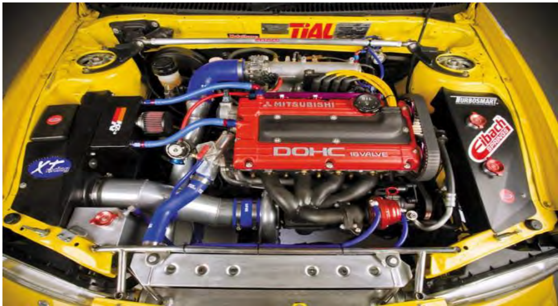
Figure 2.2 above show a forced induction engine of turbocharged engine
