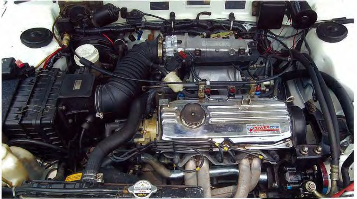
Figure 2.1 above show a naturally aspirated engine
