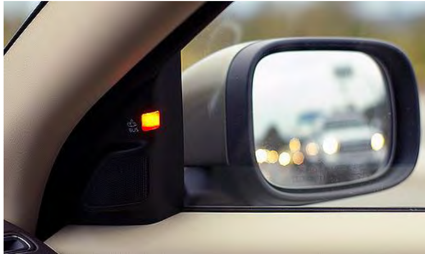
Figure 2.3: Volvo's BLIS system
