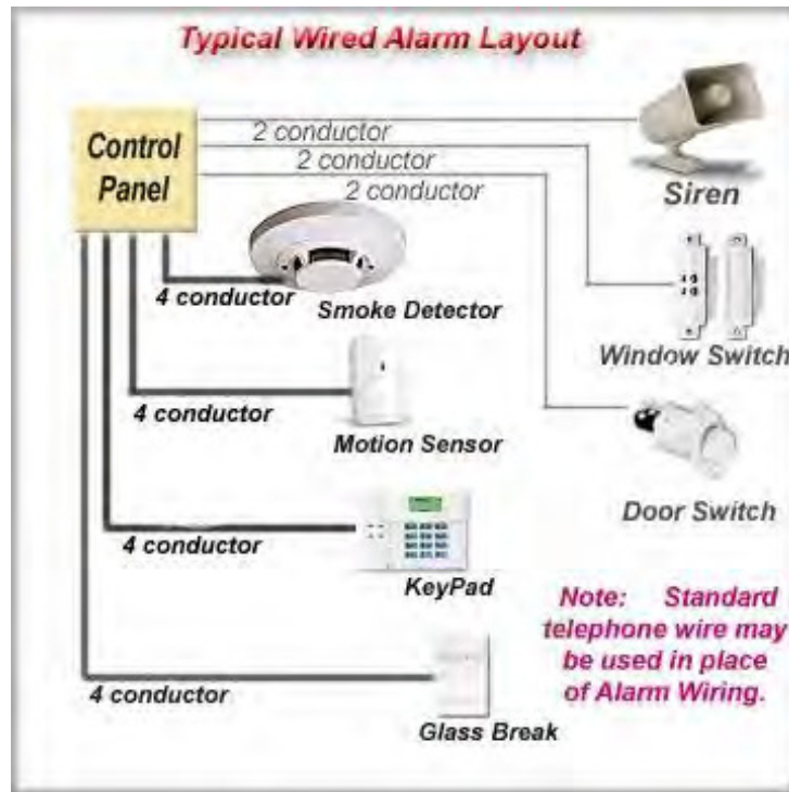
Figure 2.5: Typical Wired Alarm Layout
