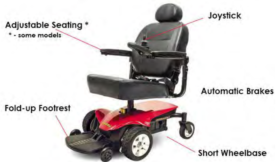
Figure 1.1 : Motorized Wheelchair And Parts
