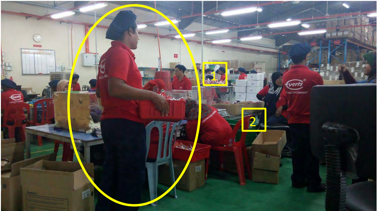
Figure 1.3: Clipping operator need to walk and manually take WIP from inner pack workstation and bring it to his workstation.
