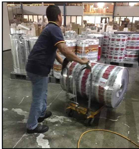
Figure 1.1: Handling of a heavy plastic roll using substandard assistive device in awkward bending posture
