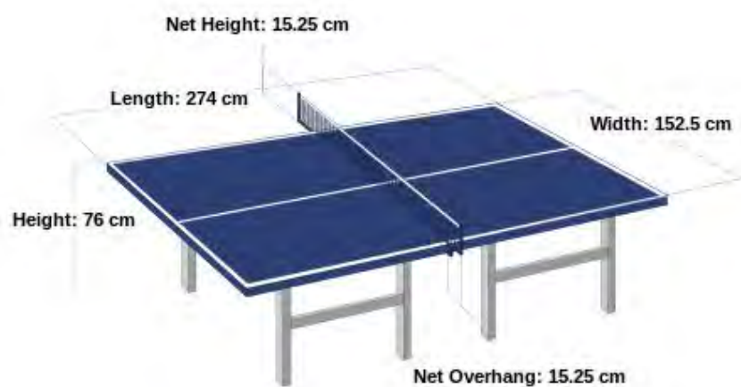
Figure 2.2: Dimensions of Table Tennis Table
