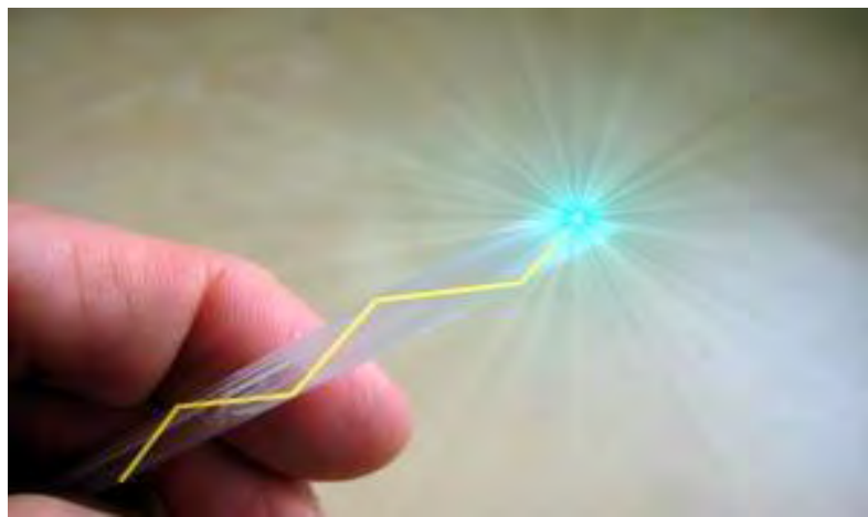
Figure 2.3: Light pipe; Optical fiber transmits the beam of light down a thin sheet of plastic or glass by making them bounce repeatedly against the wall
