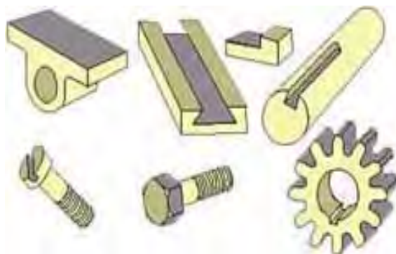
Figure 2.1: Component produced by a milling
