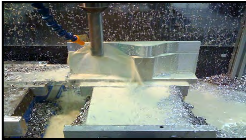
Figure 1.1: Shows cutting fluid is used on machining process.
