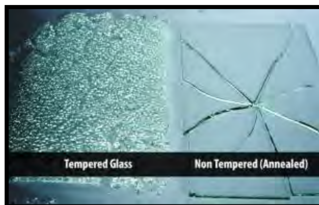
Figure 2.1: Tempered Glass versus Non-Tempered Glass
