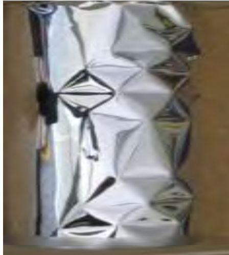
Figure 2.1: Cylindrical Shell with Elastic Buckling (Seffen & Stott, 2014)
