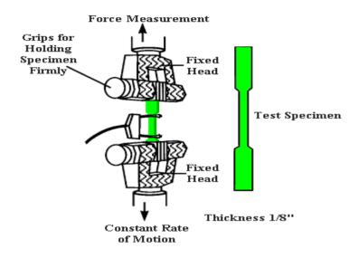
Figure 1.1:Tensile Testing
