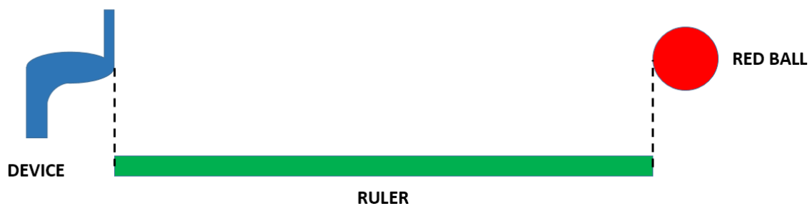
Figure 3.17: Experiment setup for distance measurement error
