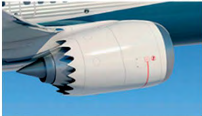
Figure 1.3: Boeing 737 MAX separate flow nacelle (Konrad, 2017).
