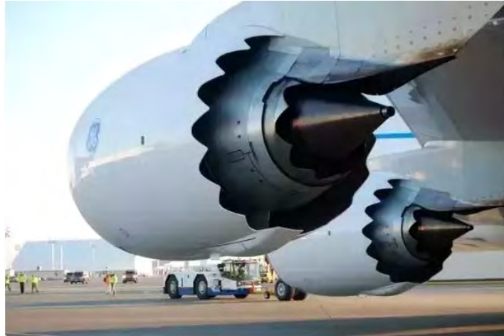
Figure 1.2: New design of exhaust nacelle in Boeing 787 (Bargsten and Gibson, 2011).
