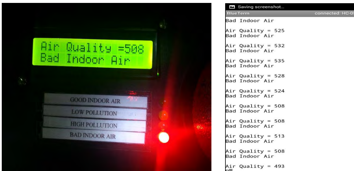
Figure 4.5: The condition change to “Bad Indoor Air” after 7 second and printed out the condition on the LCD and Smartphone application
