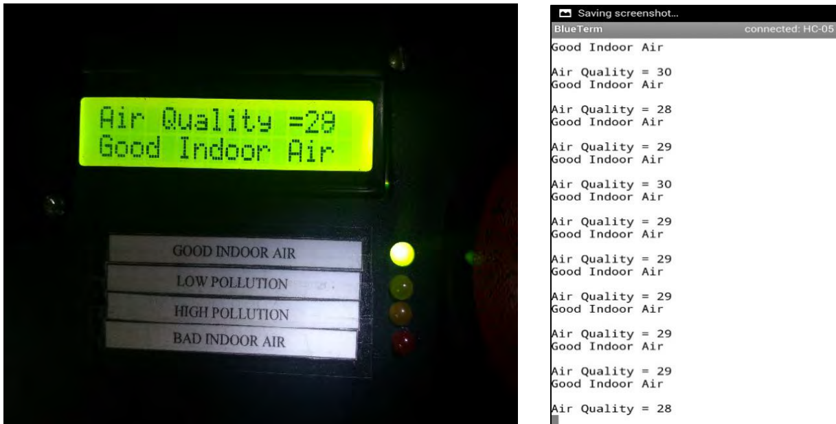
Figure 4.24: “Good Indoor Air” condition is printed out on the LCD and Smartphone application before the presence of carbon monoxide.
