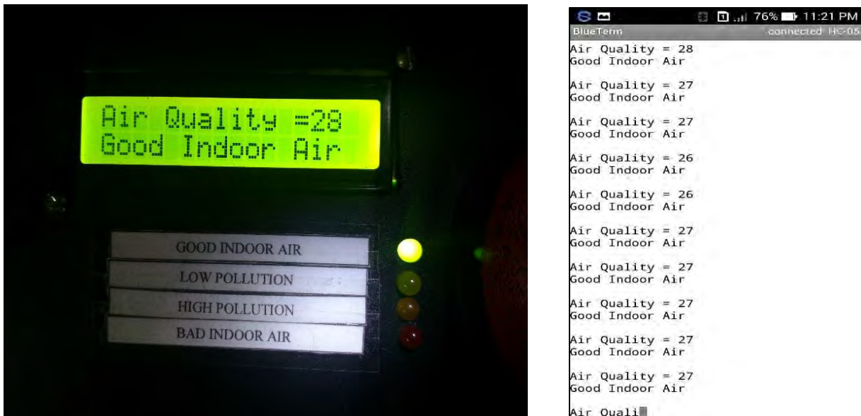
Figure 4.35: “Good Indoor Air” condition is printed out on the LCD and Smartphone application before the presence of bug spray.
