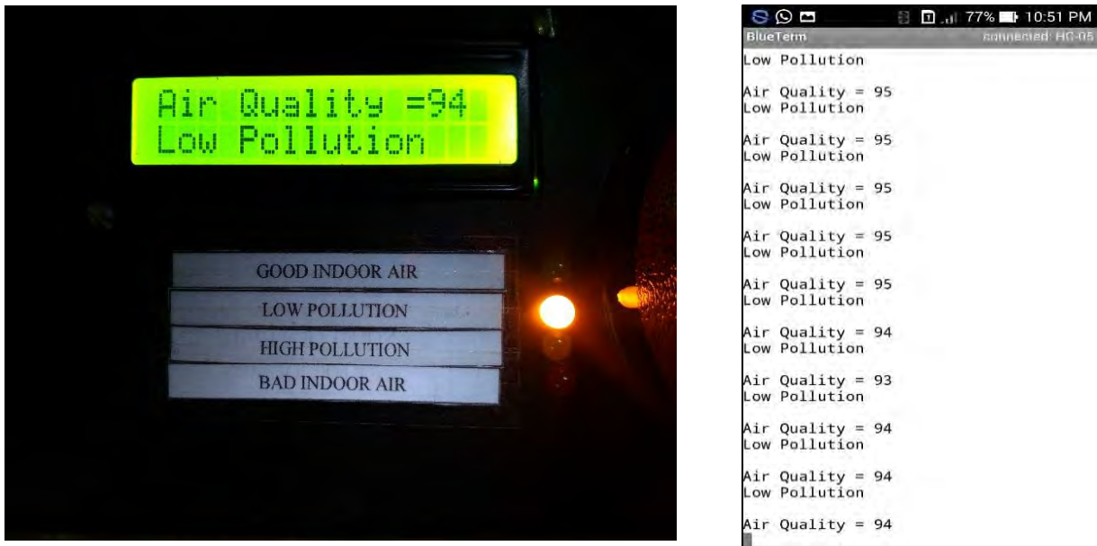
Figure 4.42: The condition change to “Low Pollution” after 3 second and printed out the condition on the LCD and Smartphone application.
