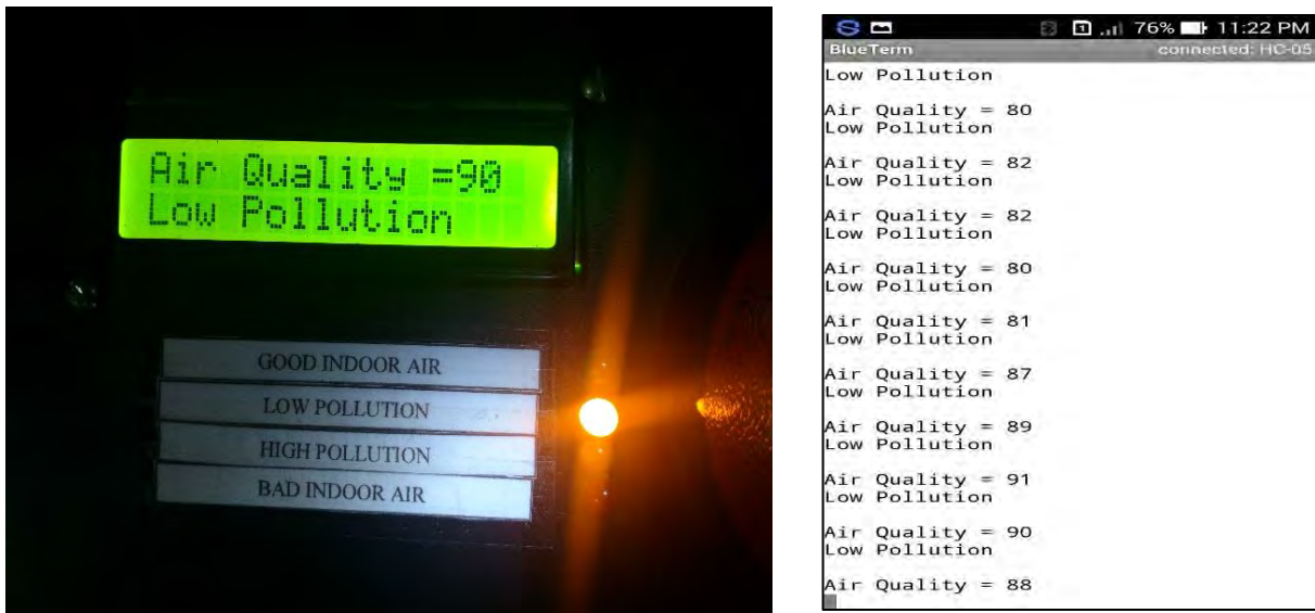
Figure 4.3: The condition change to “Low Pollution” after 3 second and printed out the condition on the LCD and Smartphone application.
