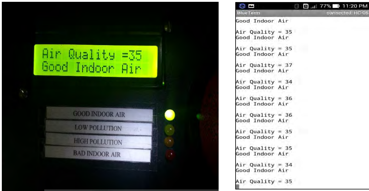
Figure 4.13: “Good Indoor Air” condition is printed out on the LCD and Smartphone application before the presence of cigarette smoke.
