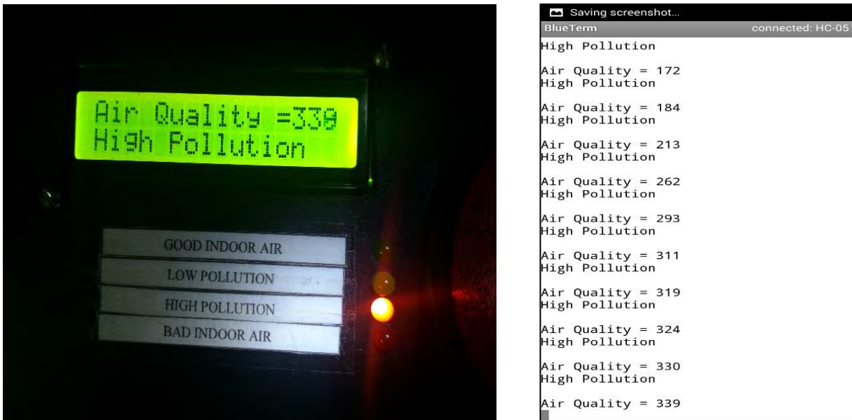
Figure 4.15: The condition change to “High Pollution” after 5 second and printed out the condition on the LCD and Smartphone application
