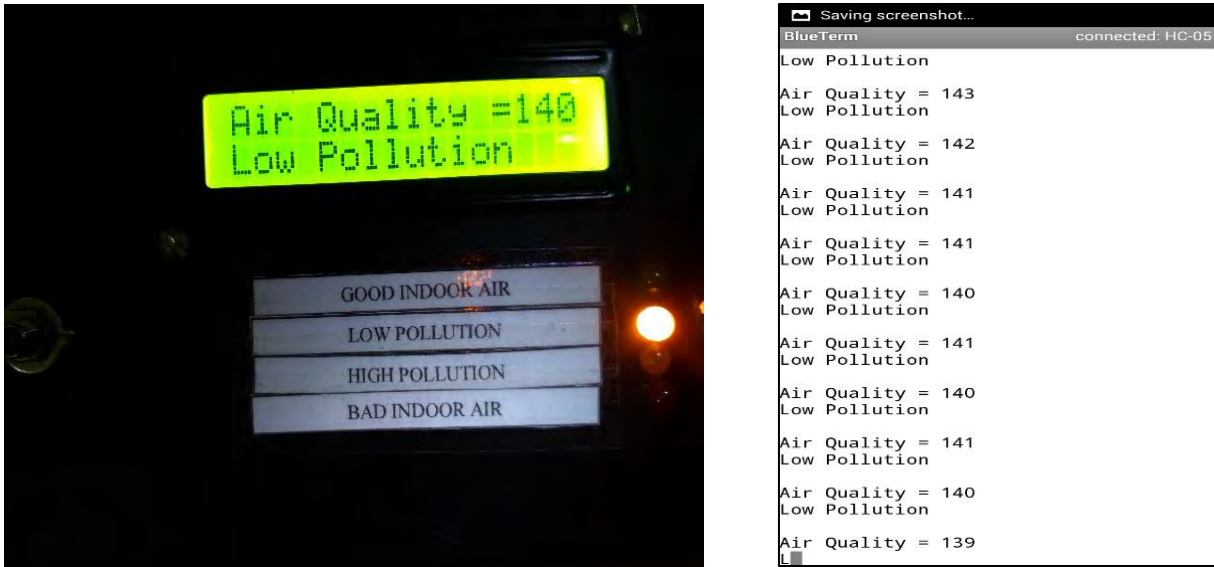
Figure 4.9: The condition change to “Low Pollution” after 3 second and printed out the condition on the LCD and Smartphone application.
