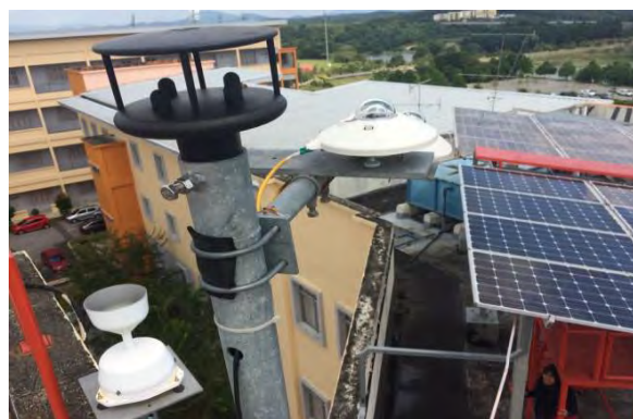
Figure 3. 4: The pyranometer install at FKE building
