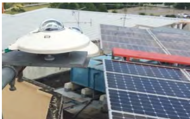
Figure 3. 8: Pyranometer designed for measuring the irradiance.
