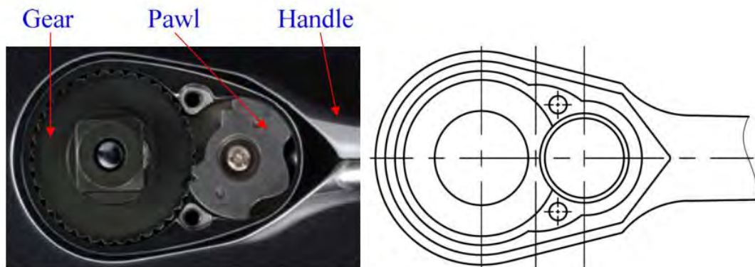
Figure 2.6: RTW with a gourd-shaped head (Chang et al., 2016)
