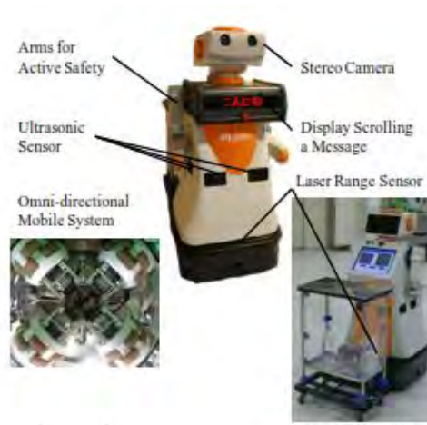
Figure 1.1 : MKR-003 *(Muratec Keio Robot) [1]
