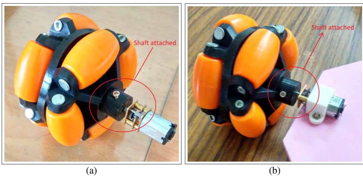
Figure 4.3: Shaft fabricated (a) combine with DC motor and Omni wheel, and (b) the combination attached to fabricated robot base.
