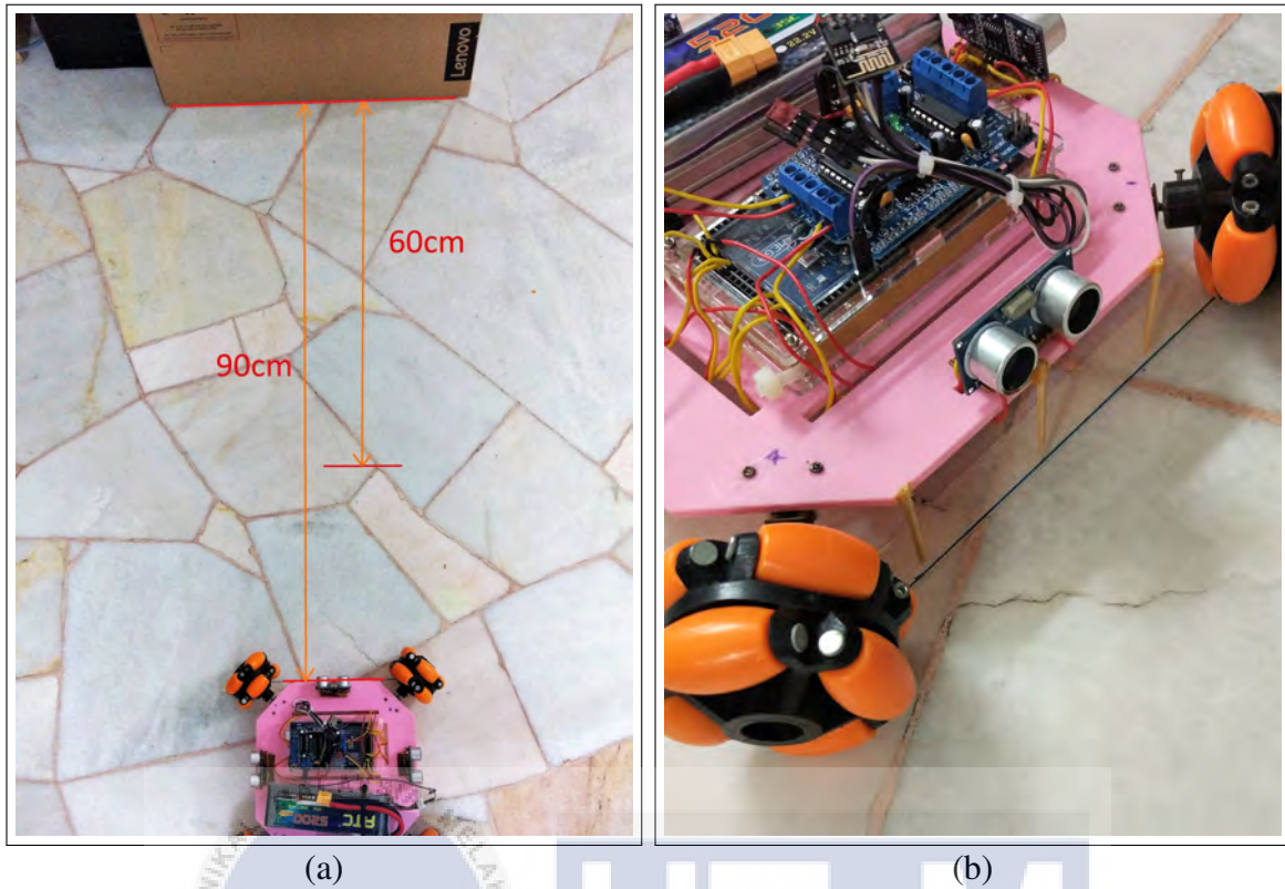
Figure 3.16: Mobile robot (a) is set-up according to 60cm and 90cm, and (b) bamboo skewer is point to the starting line.
