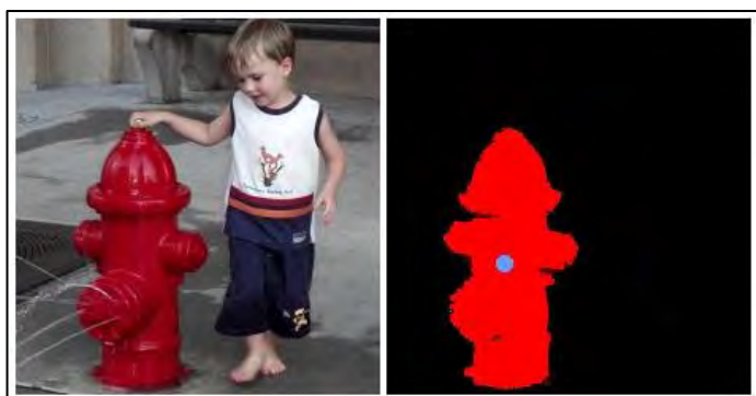
Figure 2.12: Blob detection with centre of mass of the red object [17]
