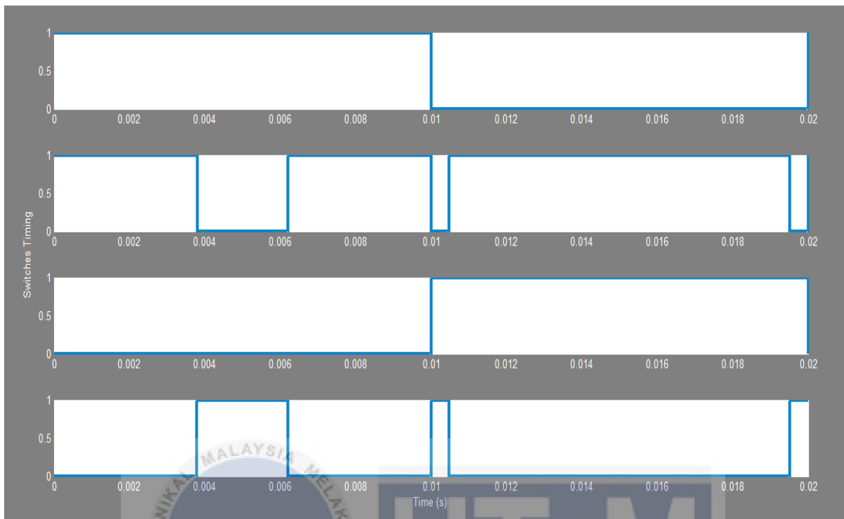
Figure 4.16(b): Lower switching waveform for non-optimization five-level CHB-MLI with MI = 0.68
