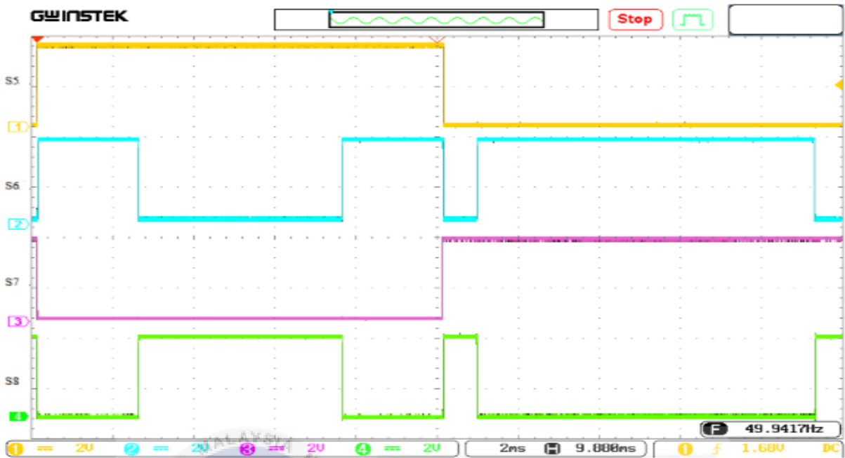
Figure 4.31(b): Lower switching waveform for optimization of five-level CHB-MLI with MI = 0.84 at \Theta_1 = 17.06^\circ and \Theta_2 = 43.53^\circ
