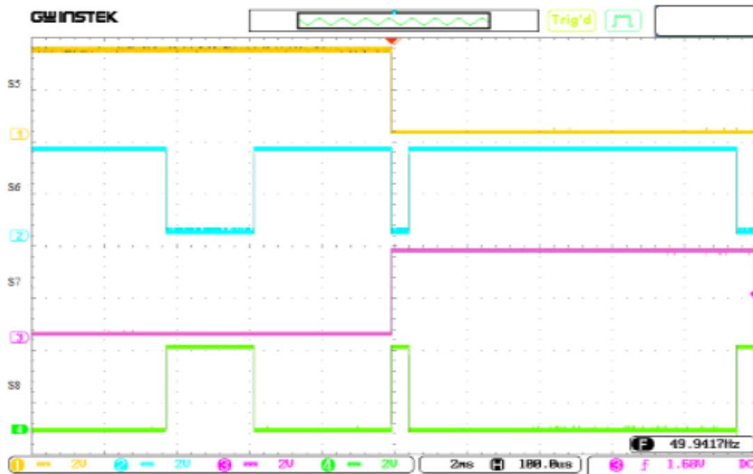
Figure 4.36(b): Lower switching waveform for non-optimization of five-level CHB-MLI with MI = 0.68 at \Theta_1 = 8.77^\circ and \Theta_2 = 68.16^\circ
