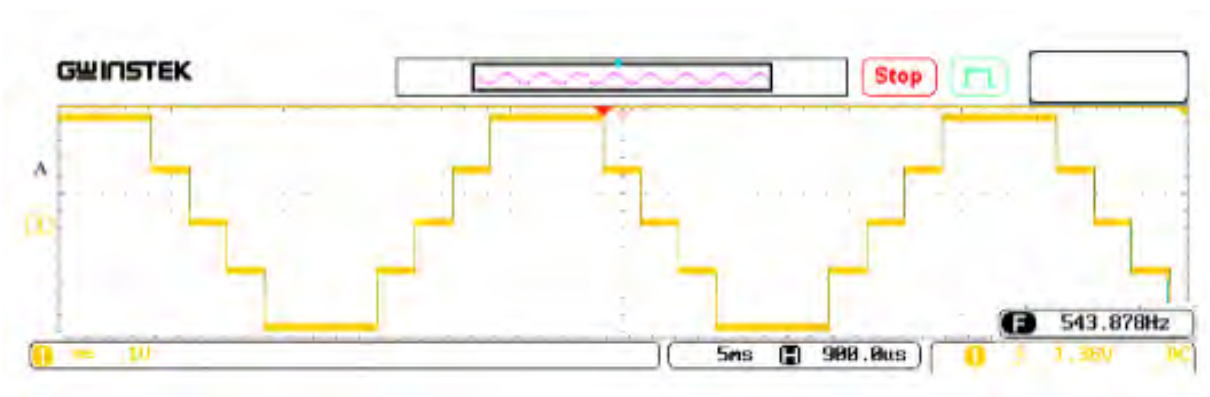
Figure 4.32: Output voltage waveform for optimization of five-level CHB-MLI
