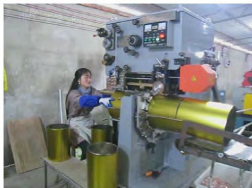
Figure 2.4: Seam Welding Machine Used in Making Container
