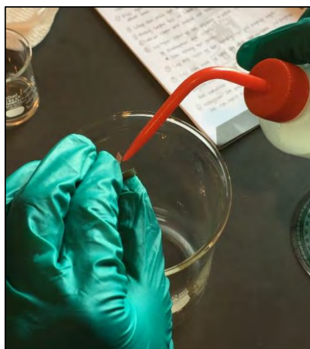
Figure 3.38: Copper strip V-shape washed with distilled water
