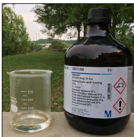
Figure 3.46: Submerge completely copper strip in 1:1 solution of HCl and distilled water
