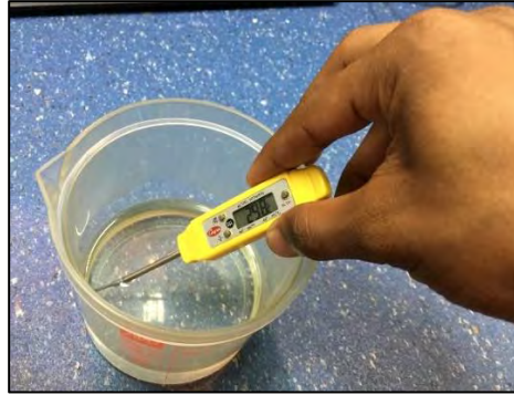
Figure 3.14: Measure initial temperature of oil sample
