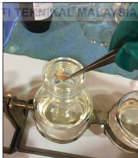
Figure 3.44: Carefully take out copper strip from heavy-walled bottle
