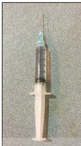
Figure 3.7: 5 ml of oil sample loaded into a syringe with needle
