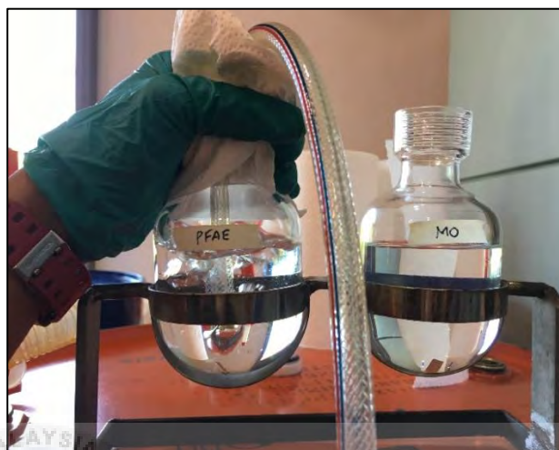
Figure 3.41: 5 minutes for bubble nitrogen through oil sample in heavy-walled bottle
