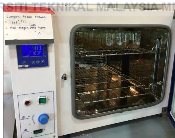
Figure 3.40: Dry copper strip V-shape in oven for 3 to 5 minutes at 80^{\circ}\text{C} to 100^{\circ}\text{C}
