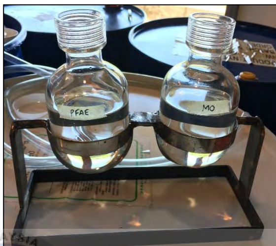
Figure 3.39: Heavy-walled bottle 250 ml are filled with 220 ml of oil sample non-filtered
