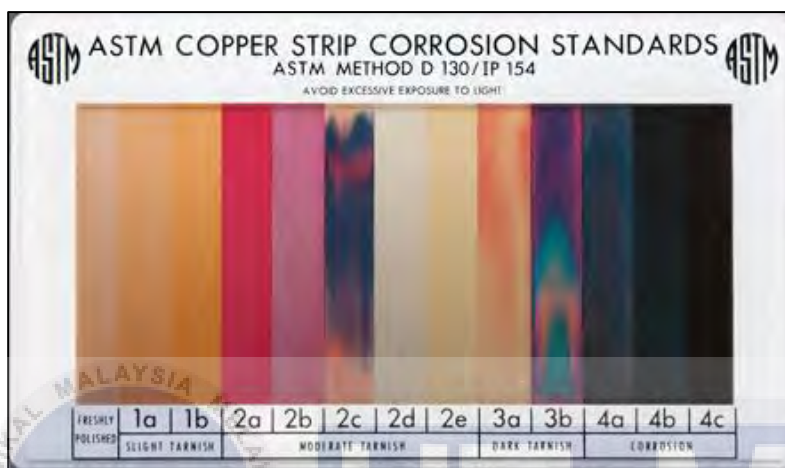
Figure 3.45: Copper strip tarnish level classification, test method ASTM D130 standards
