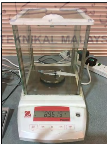
Figure 3.8: Weighing the sample inside syringe
