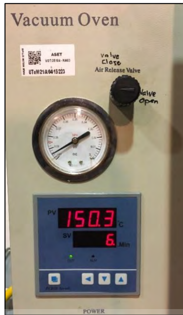
Figure 3.43: Heating heavy-walled bottle about 48 hours \pm 20 minutes at 150 \pm 2^\circ\text{C}
