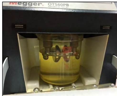
Figure 3.16: Place the oil sample in the test chamber
