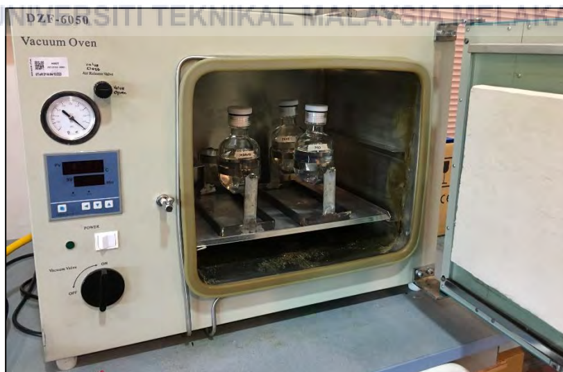
Figure 3.42: Placed heavy-walled bottle in the oven at 150°C
