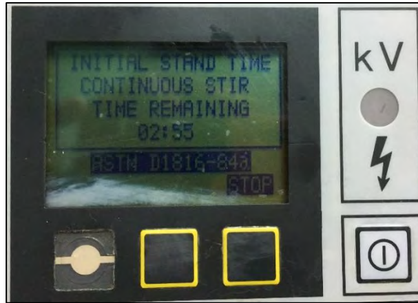
Figure 3.19: 3 minutes required for initial stirrer process
