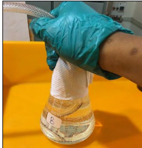
Figure 3.30: 15 minutes for bubble nitrogen through oil sample in conical flask
