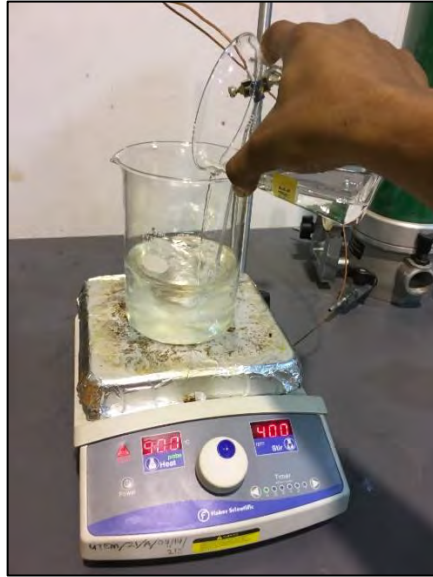
Figure 3.25: PFAE oil is poured into the beaker when temperature is reached 90°C
