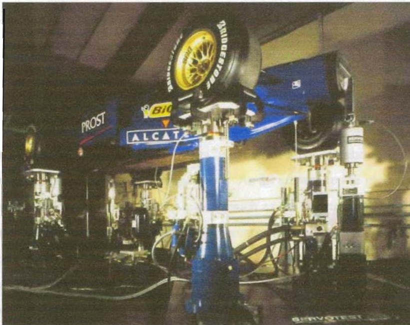
Figure 1: Image of ServoTest 7-post Test Rig
