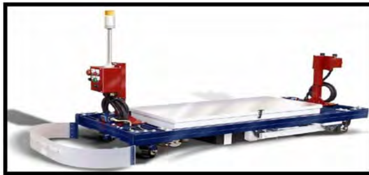
Figure 2.4: Automatic Guided Cart (AGC) [6]
